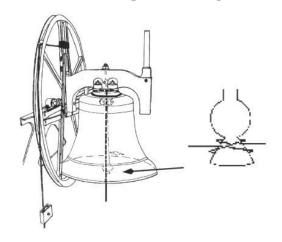
Twist the loop round so that the long end of the rope hangs down on the far side of the bell.
