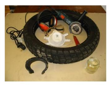
Fig 1 shows what's needed, apart from a piece of chalk, which I forgot, and my trusty old Black & Decker Workmate, which wouldn't fit in the picture. On the left is the safety gear: mask, goggles and ear defenders. The only tools required are a mini-disk angle grinder and a Stanley knife with a new blade. Some might feel happier to include a tape measure even though it isn't necessary, but the jar of water certainly is!
