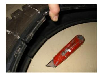
In Fig 3 you can see the two cuts through the wire reinforcing of each rim. If you were making a complete set, you would mark up all the cuts before starting to use the grinder; so all this noisy filthy work can be completed in one go. Having removed the tyre from the workmate you can now cut around the marks with the Stanley knife, dipping the blade frequently in the water. Why? Try cutting with a dry knife and you'll find out!
