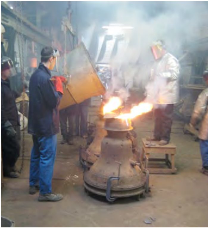
Casting the treble and 2 at Whitechapel.
